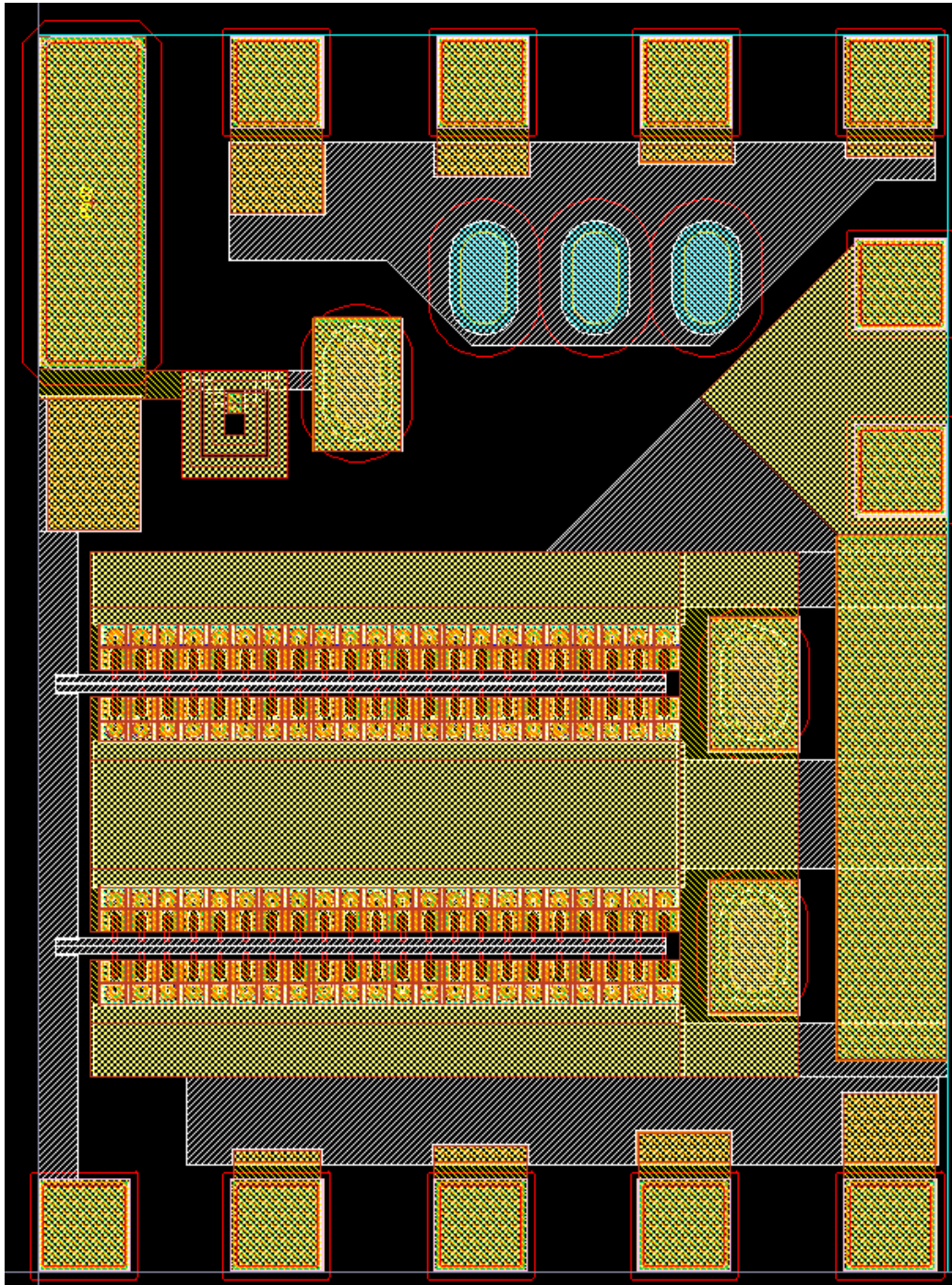
Figure 4.23: Layout of common emitter chip with 88 HBTs in parallel
