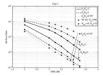
Fig. 7: Performance comparison : Type-1 Receiver.
