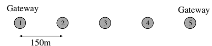
Fig. 8. Line topology: the nodes are 150 m apart. The edge nodes 1 and 5 act as gateway nodes, with all the calls being routed through them.
