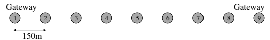
Fig. 18. Nine node line topology: the edge nodes 1 and 9 act as gateway nodes.
