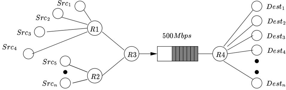
Fig. 4. Y-shape multi-queue topology with 4 different propagation delays.
