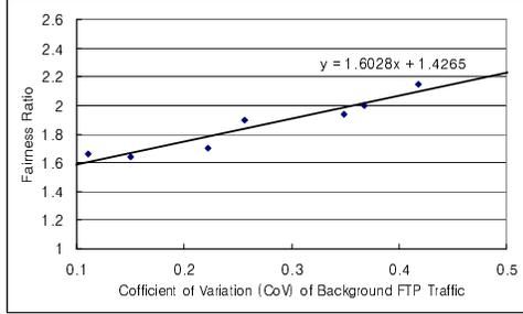
Fig. 7. Coefficient of Variation of FTP background traffic vs. Fairness Ratio
