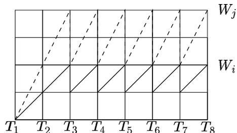
Fig. 3. Congestion window sizes of 2 synchronized TCP flows.
