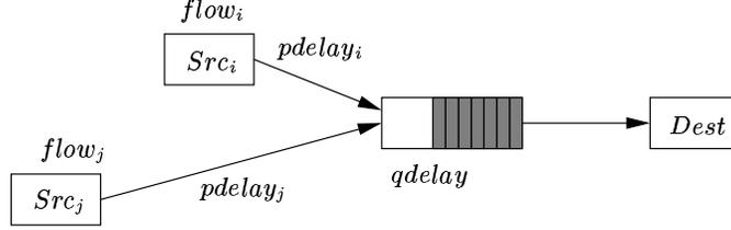
Fig. 2. Topology with two TCP flows with different propagation delays
