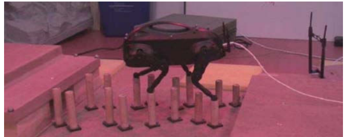
Fig. 1. LittleDog demonstrates careful foot placement.
