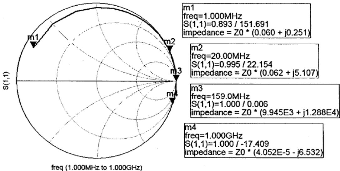
3. A shorted transmission line stub was measured on the network analyzer up to 2 GHz. From the data provided, determine the  $Z_0$ , phase velocity and effective dielectric constant of the transmission line. The physical length is 2 cm.
