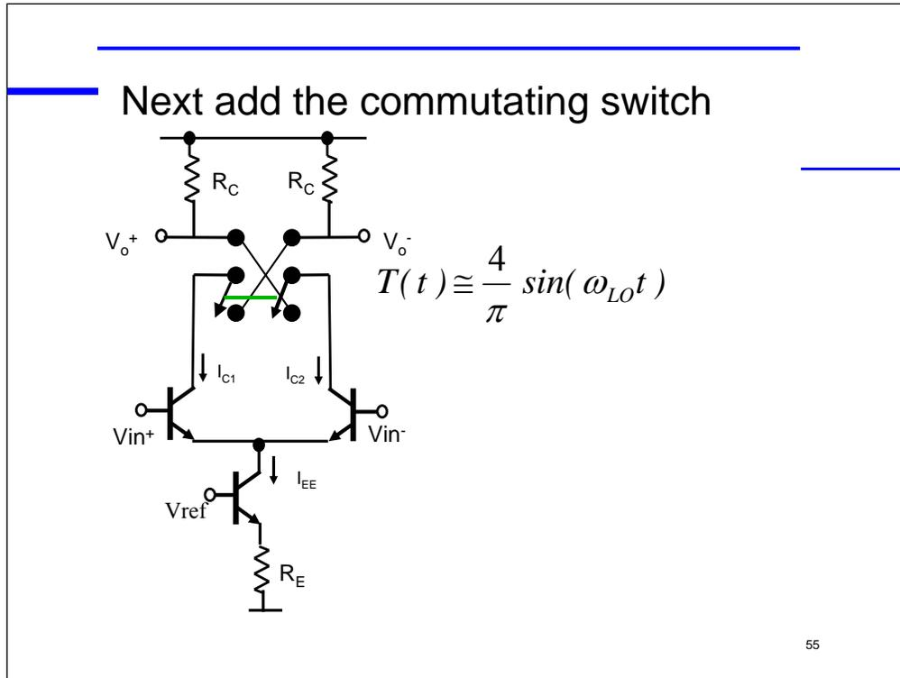
If we neglect higher order terms in the switch function, it is easy to estimate the voltage gain. Simply multiply the switch function  $T(t)$  and the small signal gain of the diff pair:
