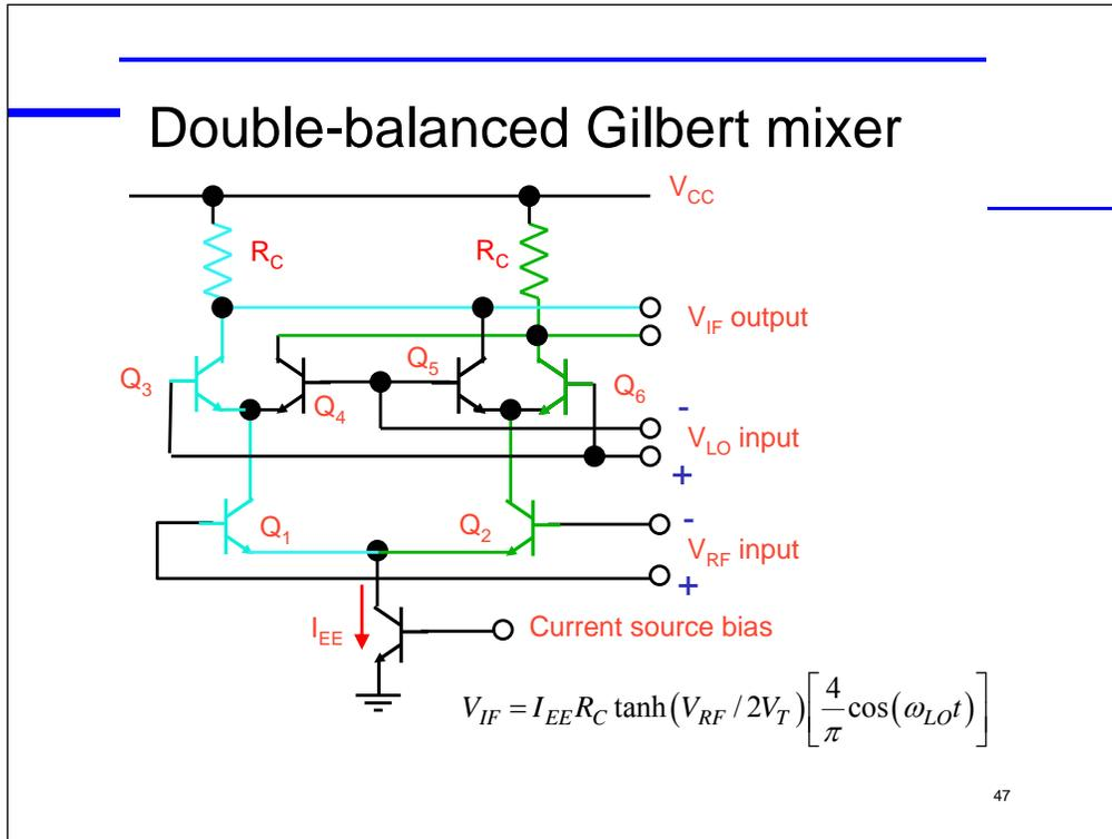
Suppose that more RF current is flowing through Q1 (blue) and less through Q2 (green) and LO transistors Q3,Q6 are fully on. We see that the differential current path causes green to have higher output voltage than blue.
