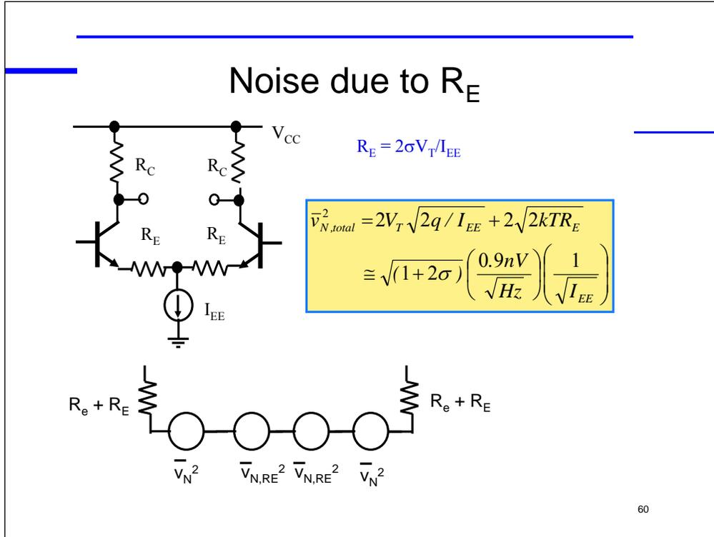
We saw that the emitter degeneration made a big difference in the upper end of the dynamic range. But, it will also increase the noise at the input, raising the noise floor. We can estimate how much the noise will be increased by the emitter resistors. Adding two resistors  $R_E$  in the base-emitter loop will introduce a thermal (Johnson) noise spectral density of  $\sqrt{2} (4kTR_E)^{1/2}$ . This is equal to
