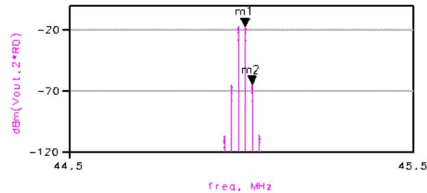
Third-order intermodulation products at  $2f_1 - f_2 - f_{LO}$  and  $2f_2 - f_1 - f_{LO}$  will be present in the IF output.
