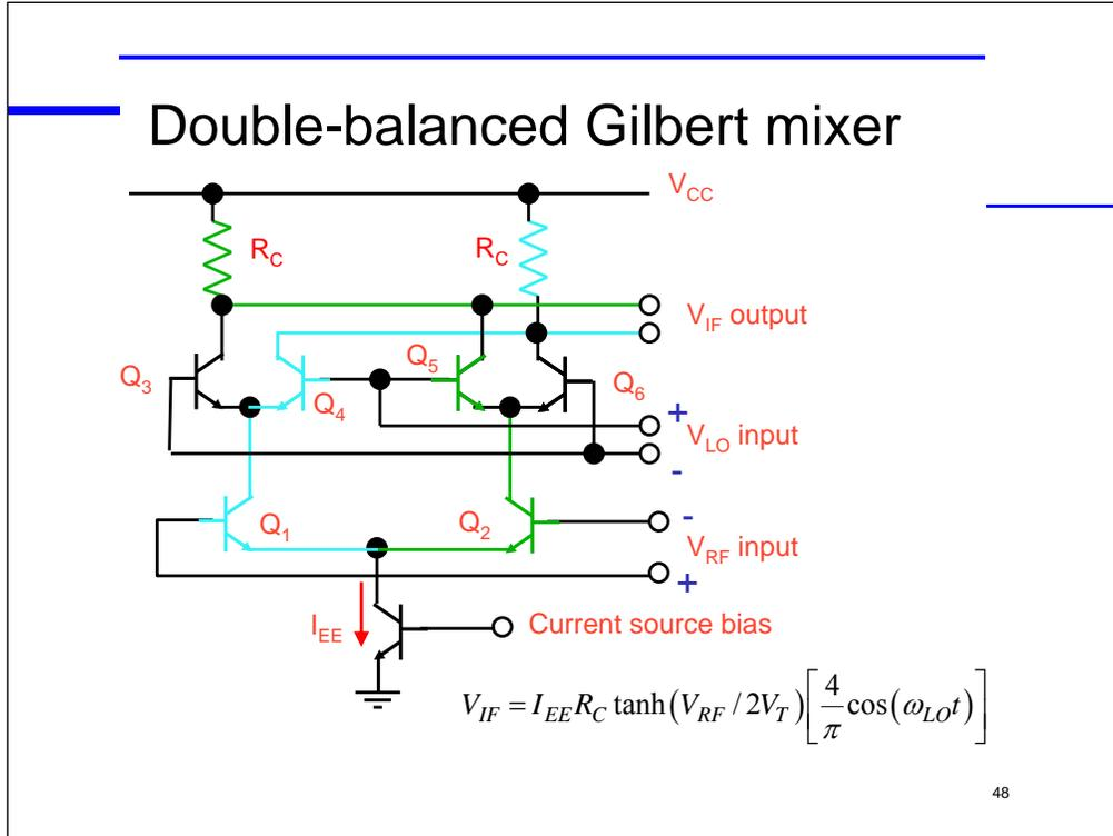
Suppose that more RF current is flowing through Q1 (blue) and less through Q2 (green) and now LO transistors Q4, Q5 are fully on. We see on this LO half cycle that the differential current path causes green to have lower output voltage than blue.
