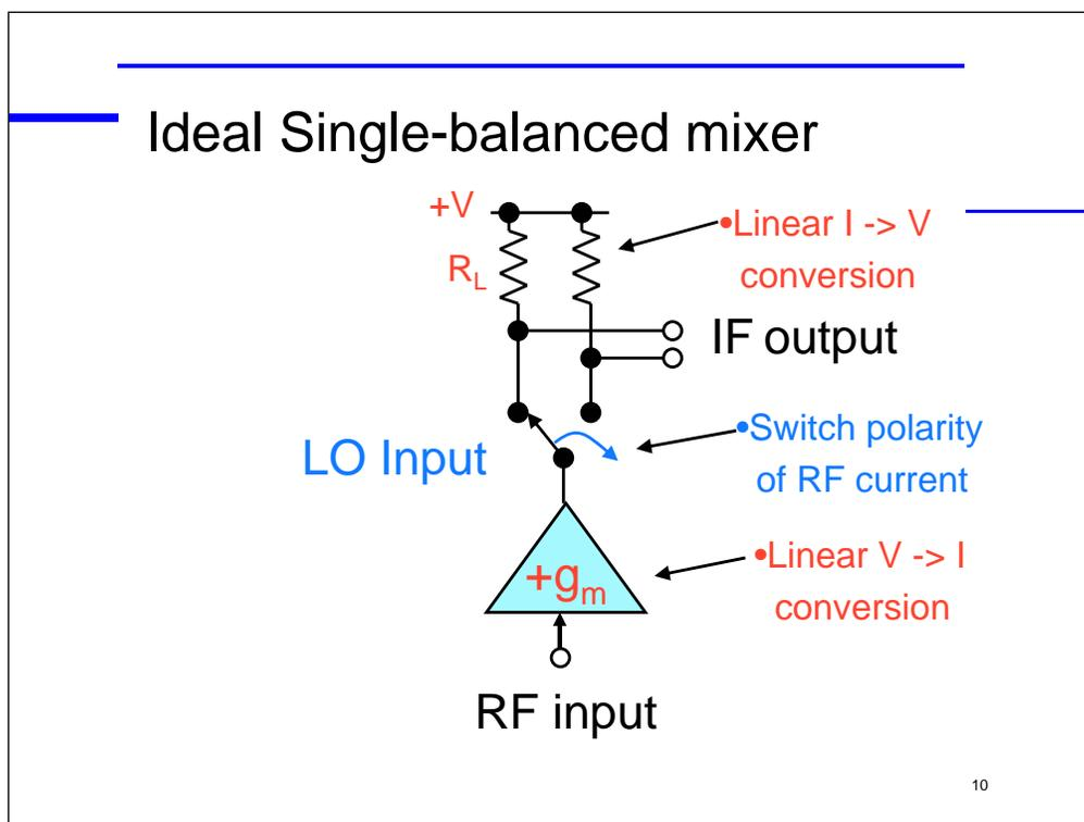
The RF feedthrough can be eliminated by using a differential IF output and a polarity reversing LO switch.
