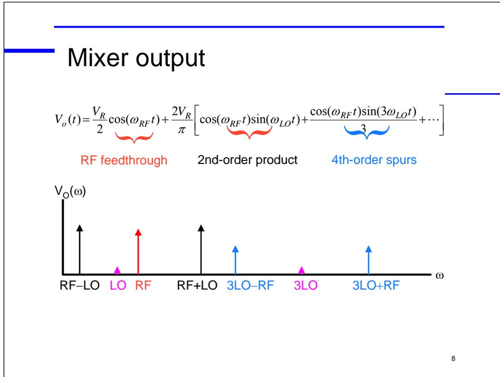
The product of  $V_{RF}(t)T(t)$  produces the desired output frequencies at
