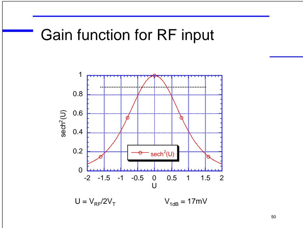
Gain drops 10% for inputs as small as  $U = \pm 0.33$ . This corresponds to an amplitude of only 17 mV and is approximately the 1 dB compression input voltage. This is  $-19$  dBm in a 50 ohm system.
