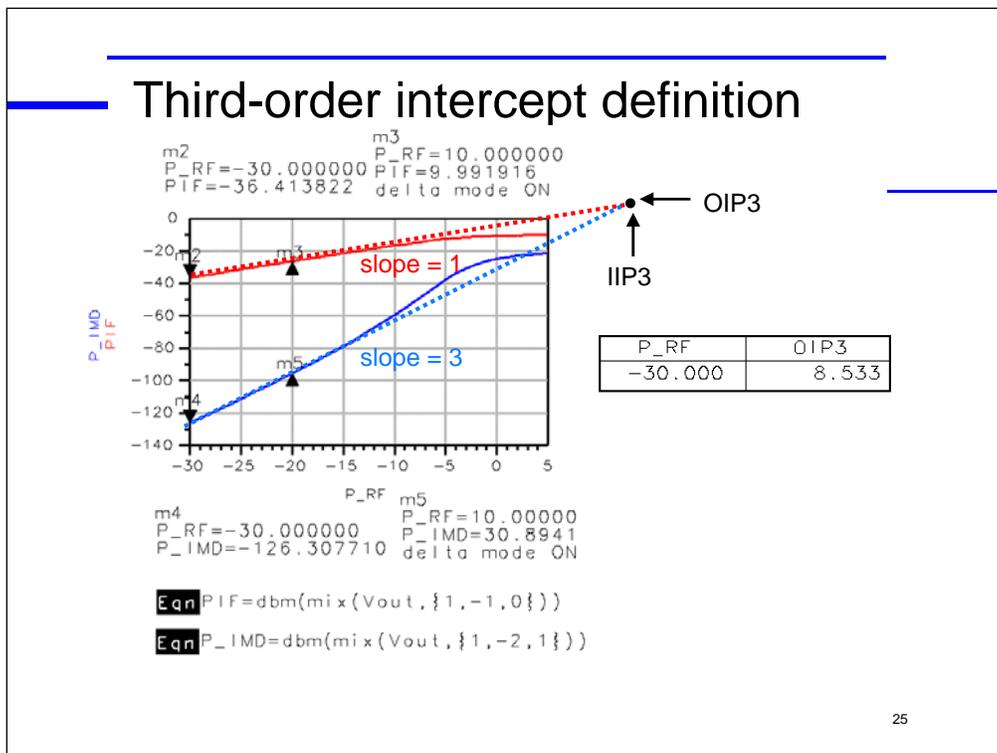
A widely-used figure of merit for IMD is the *third-order intercept* (TOI) point. This is a fictitious signal level at which the fundamental and third-order product terms would intersect. In reality, the intercept power is 10 to 15 dBm higher than the P<sub>1dB</sub> gain compression power, so the circuit does not amplify or operate correctly at the IIP3 input level. The higher the TOI, the better the large signal capability of the mixer.
