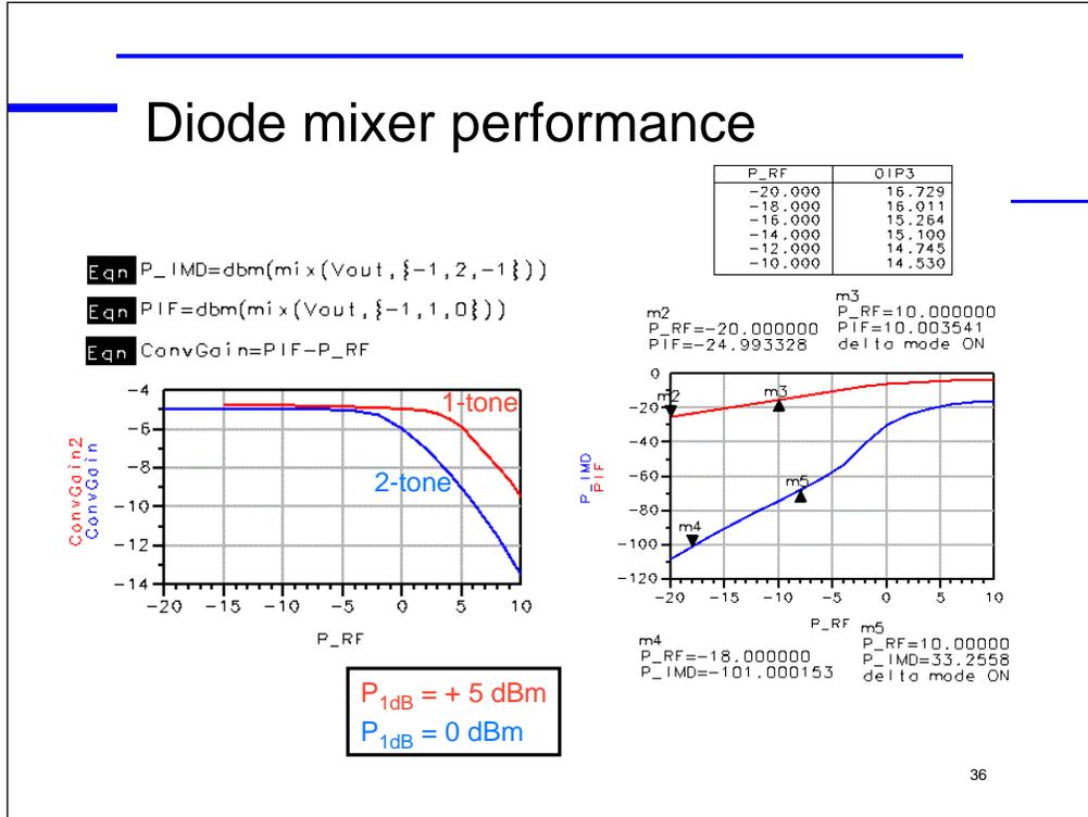
A harmonic balance simulation can be used to estimate the mixer performance. With the DB diode mixer, the currents in the diodes are half wave, so a high number of LO harmonics and maximum order and some oversampling of the FFT operation are necessary to reproduce this waveform and therefore get reasonable accuracy on the third-order product. Gain compression is not as sensitive to the LO order.
