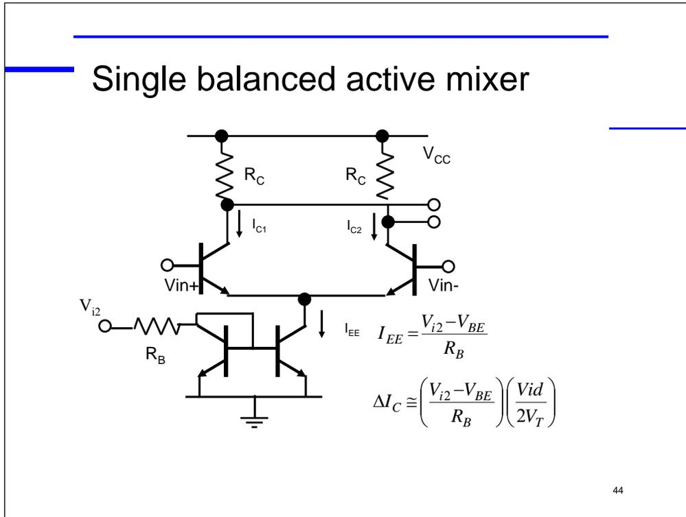
But,  $V_{i2} > V_{BE}$  and  $V_{id}$  must be small,  $\ll V_T$ . Rather limited use.
