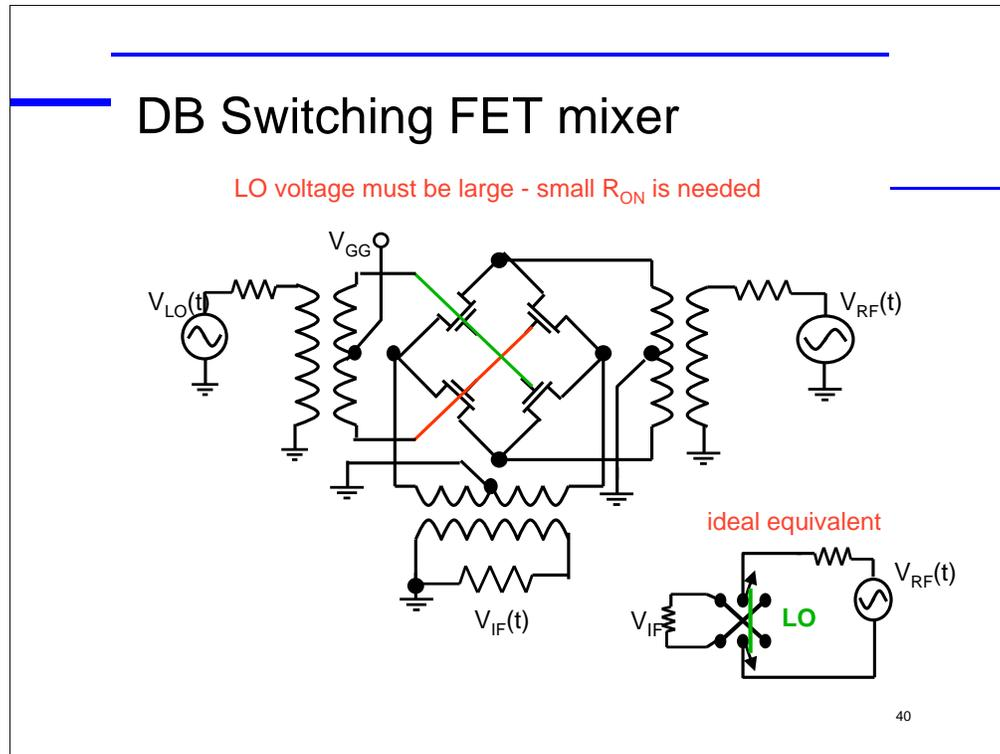
The channel resistance of a large FET when in its triode region (below saturation) can be quite low and is not as current dependent as the diode. Therefore, switching configurations using FETs can be more linear in the RF to IF path than diode switching mixers.
