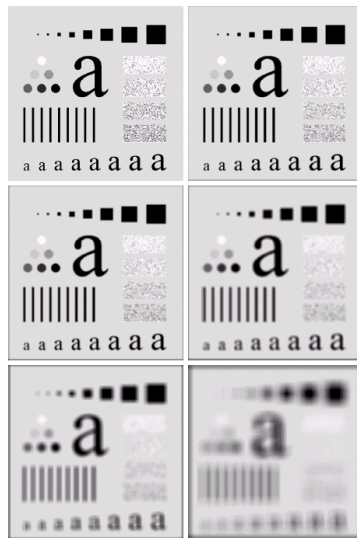
FIGURE 3.35 (a) Original image, of size 500 \times 500 pixels. (b)–(f) Results of smoothing with square averaging filter masks of sizes n = 3, 5, 9, 15, and 35 , respectively. The black squares at the top are of sizes 3, 5, 9, 15, 25, 35, 45, and 55 pixels, respectively; their borders are 25 pixels apart. The letters at the bottom range in size from 10 to 24 points, in increments of 2 points; the large letter at the top is 60 points. The vertical bars are 5 pixels wide and 100 pixels high; their separation is 20 pixels. The diameter of the circles is 25 pixels, and their borders are 15 pixels apart; their gray levels range from 0% to 100% black in increments of 20%. The background of the image is 10% black. The noisy rectangles are of size 50 \times 120 pixels.
