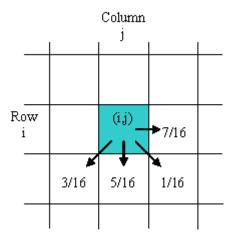
Quantization error observed at pixel (i, j) is diffused to the right, lower left, below and lower right pixels with the following weights (7/16, 3/16, 5/16, 1/16). Here, note that the weights sum up to 1.
