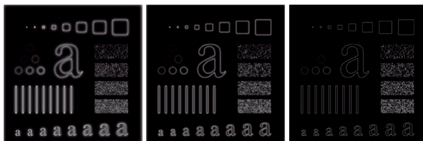
FIGURE 4.26 Results of highpass filtering the image of Fig. 4.11(a) using a GHPF of order 2 with D_0 = 15 , 30, and 80, respectively. Compare with Figs. 4.24 and 4.25.
