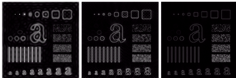
FIGURE 4.24 Results of ideal highpass filtering the image in Fig. 4.11(a) with D_0 = 15 , 30, and 80, respectively. Problems with ringing are quite evident in (a) and (b).
