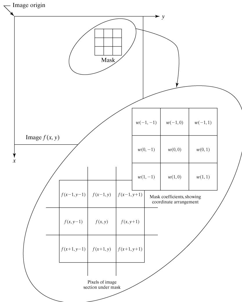
**FIGURE 3.12** The mechanics of linear spatial filtering. The magnified drawing shows a  $3 \times 3$  mask and the corresponding image neighborhood directly under it. The neighborhood is shown displaced out from under the mask for ease of readability.
