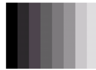
FIGURE 2.7 (a) An example showing that perceived brightness is not a simple function of intensity. The relative vertical positions between the two profiles in (b) have no special significance; they were chosen for clarity.
