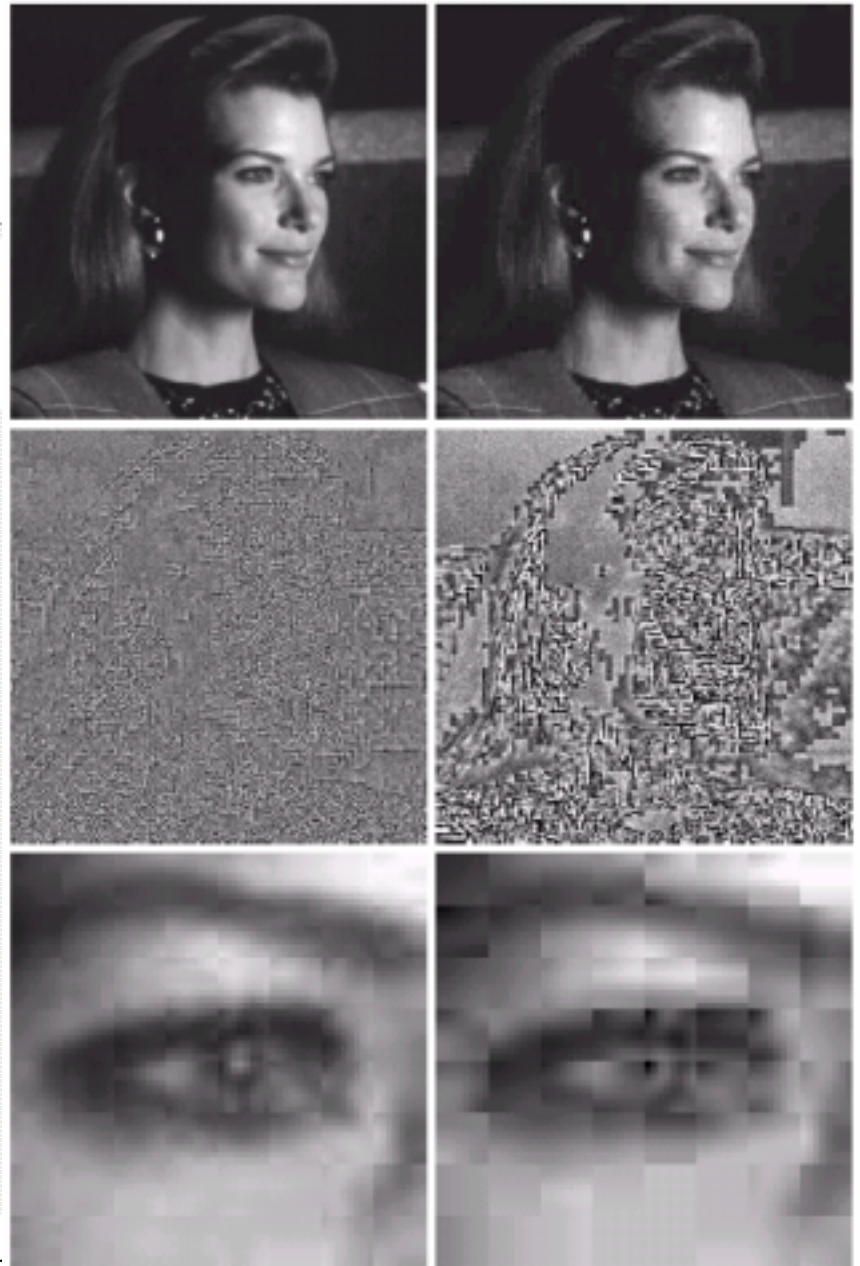
FIGURE 8.38 Left column: Approximations of Fig. 8.23 using the DCT and normalization array of Fig. 8.37(b). Right column: Similar results for 4Z .
