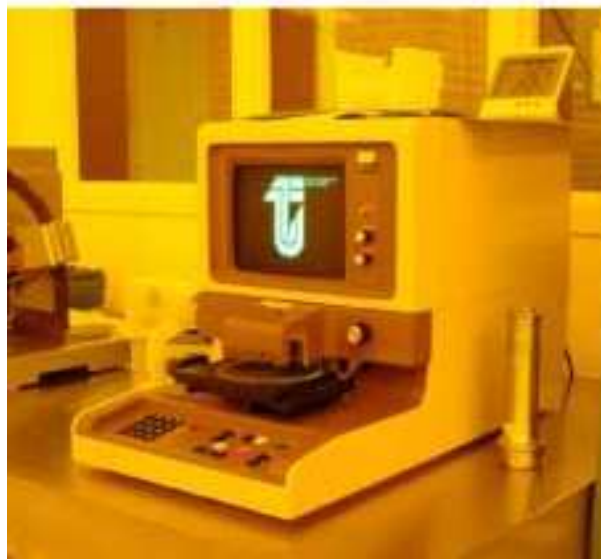
Figure E.17: Tencor Alphastep 200 used to measure the etch depth.
