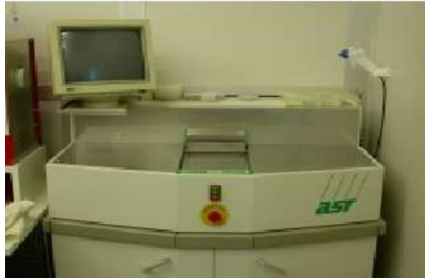
Figure E.8: Rapid Thermal Annealing machine used for annealing.
