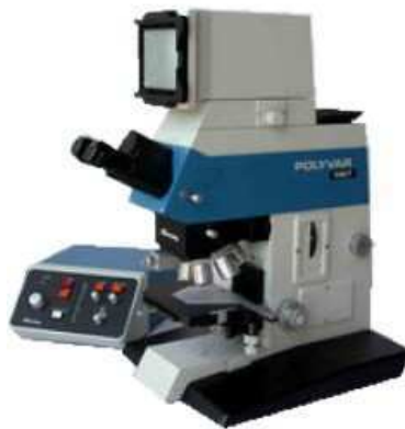
Figure E.2: Optical Microscope (Reichert Jung Polyvar) used to check the structure on the sample.
