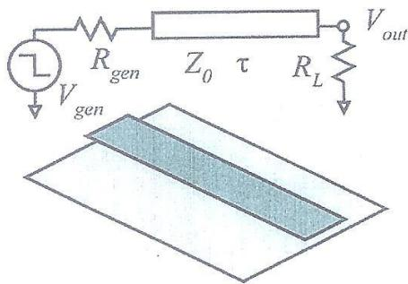
Approximate the effect of fringing fields at the edges of the conductors by assuming that the effective microstrip line width is the physical width plus twice the conductor-ground spacing.
