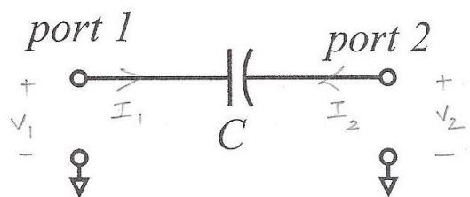
Z-Parameters ;  $Z_{11} = \frac{v_1}{I_1} \Big|_{I_2=0}$
