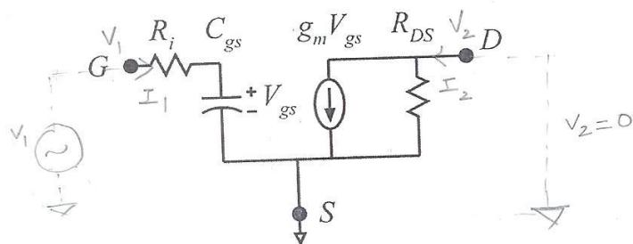
$$Y_{11} = \frac{I_1}{V_1} \Big|_{V_2=0}$$
