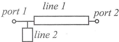
Approximate the effect of fringing fields at the edges of the conductors by assuming that the effective microstrip line width is the physical width plus twice the conductor-ground spacing.
