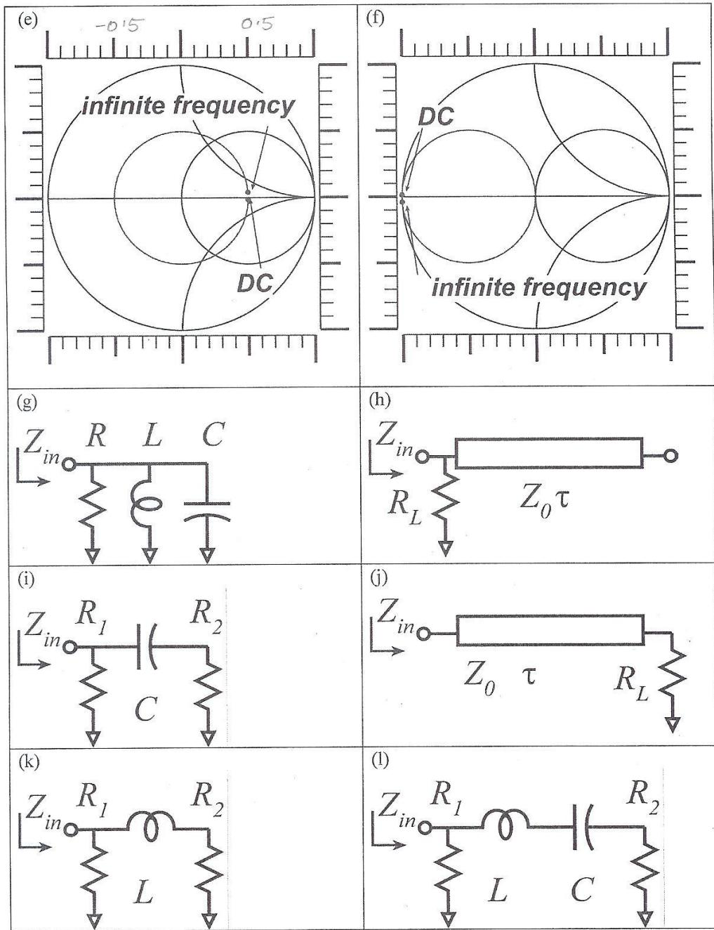
First match each Smith Chart with each circuit. Then determine as many component values as is possible (RLC values, transmission line delays and characteristic impedances)...note that some values cannot be determined with the information given.
