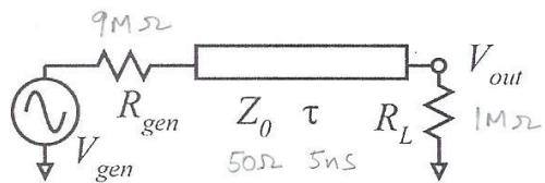
What is the -3dB frequency of this test setup?
