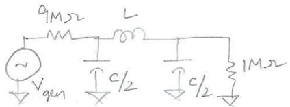
$$5 \quad \tau_{LR} = \frac{L}{R_{\text{gen}} + R_L} \\ = \frac{250 \text{ nH}}{9 \text{ M}\Omega + 1 \text{ M}\Omega} \\ \boxed{\tau_{LR} = 25 \text{ fs}}$$
