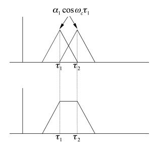
[**Delay Spread**] Send a signal with length T and channel  $\tau_{\text{max}} - \tau_{\text{min}} = T_m$ . The output length is  $T + T_m$ . It causes ISI.
