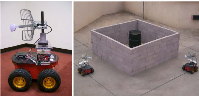
Fig. 3. (left) A pioneer 3-AT robot equipped with our servo control mechanism/fixture and an adaptive narrow-beam directional antenna and (right) two robots in action on our campus, making wireless measurements in order to map the obstacle.
