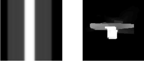
Fig. 5. Comparison of our mapping framework in the reconstruction of the T-shaped structure of Fig. 4, at 0.77% sampling rate, with (left) coordinated samples distributed over one angle and (right) random sampling.
