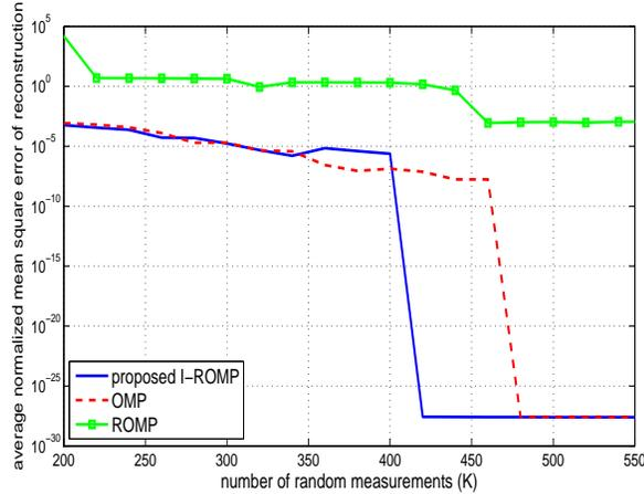
Fig. 5. Reconstruction of the sparsified signal of Fig. 4 based on an incomplete observation set using compressed sensing (length of  $X$  is  $N = 4096$ ).
