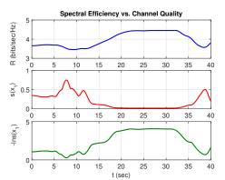
Fig. 4: (Top) The robot's spectral efficiency; (Middle) The predicted channel quality metric; (Bottom) The negative log of the predicted channel quality metric for a better comparison with the spectral efficiency. Overall, the figure confirms the results of Theorem 1.
