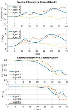
Fig. 6: The spectral efficiencies and the negative log of the predicted channel quality metric along the optimal paths. The top figure shows the results for Agents 2, 4, and 5. The bottom figure shows the results for Agents 1, 3, and 6. The results validate Theorem 1.
