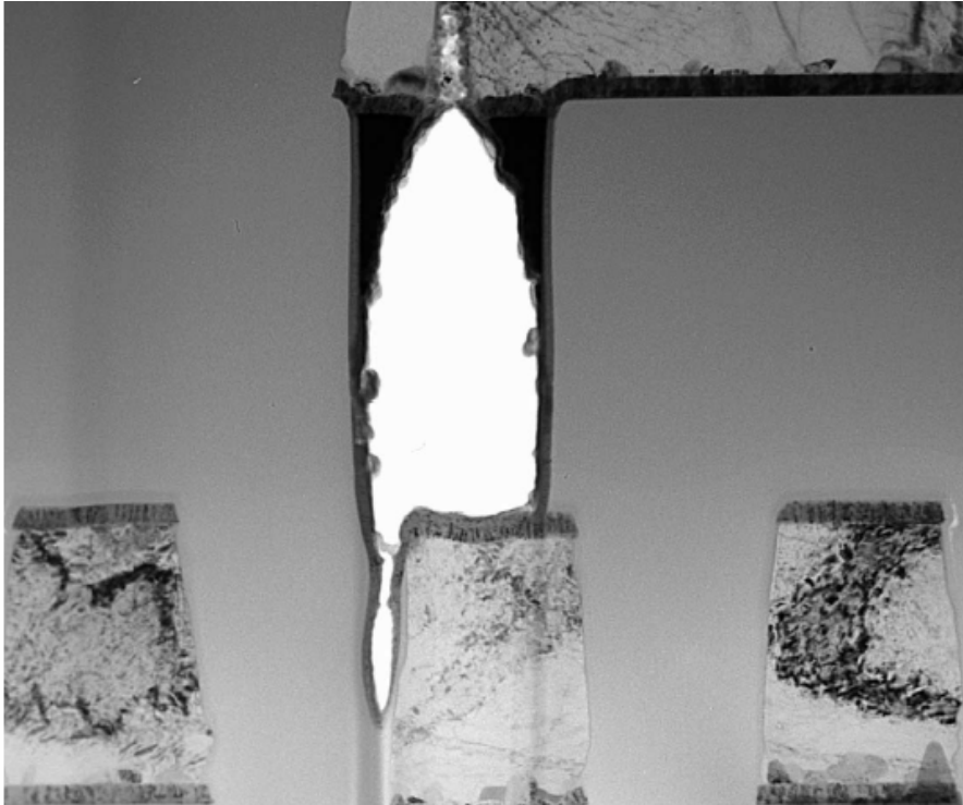
Resistive open due to unfilled via [R. Madge et al., IEEE D&T , 2003]
