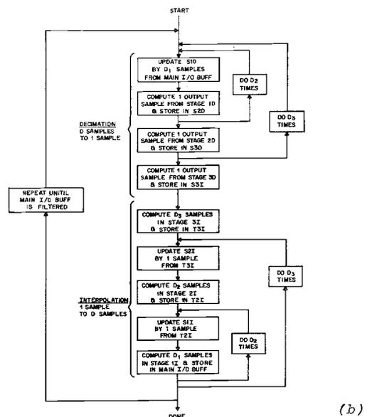
Figure 6: (a) A block diagram for implementation of a three-stage decimator followed by a three-stage interpolator, and (b) its control sequence.
