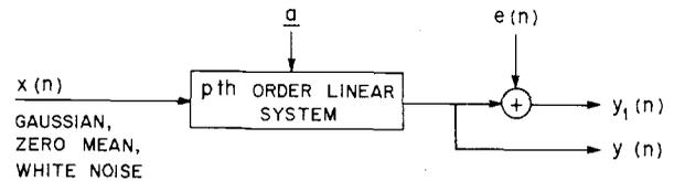
Fig. 1. Block diagram of system used to investigate log likelihood ratio distances for LPC coefficients.
