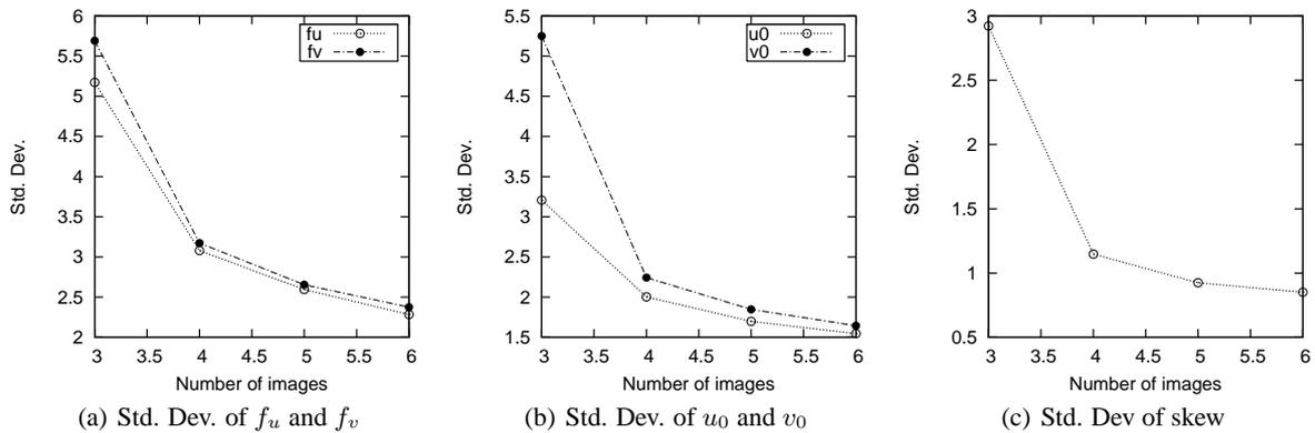
Figure 6: Effect of increasing the number of images on calculating intrinsic parameters
