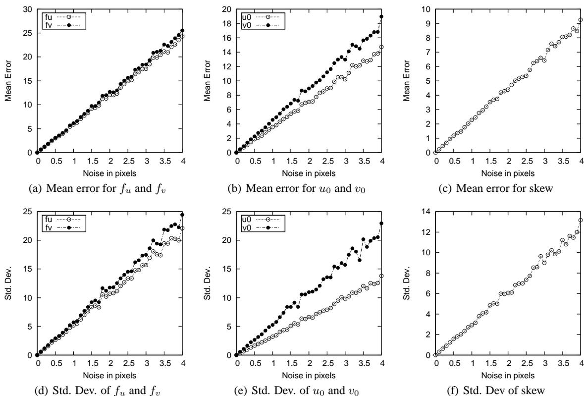
Figure 5: Influence of noise in calculating intrinsic parameters
