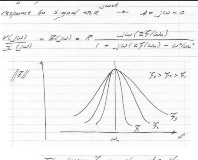
The larger & is, the wider the resonant peak in Frequency.
