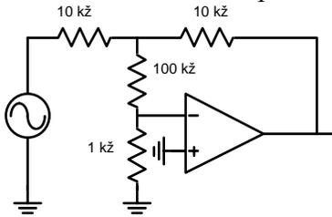
In the circuit to the right, apply an AC input signal as indicated and measure the amplifier output voltage and the voltage at the junction of the two 10 kΩ resistors (call this  $V_x$ ). The amplifier gain is then 101 times  $V_{out}/V_x$ .
