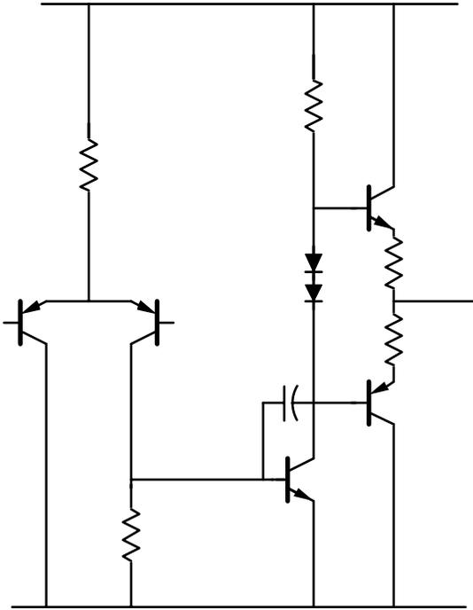
This is possibly the simplest possible OP-AMP configuration. You may be able to meet the design specification with this design. On the other hand, once you know how to design multistage circuits, it is actually easier to meet 'specs with a design with more transistors.
