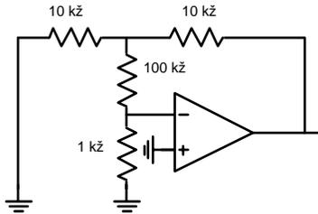
The DC output voltage will be about 200 times the input offset voltage.
