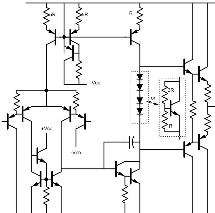
This illustrates some more tricks: Emitter followers are used in the current mirrors to eliminate base-current errors, and a Darlington input stage is used to increase the amplifier differential input impedance and to decrease the amplifier input bias current (base current).
