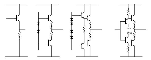
The third stage, the output stage, is almost always some kind of compound emitter follower stage. A few are illustrated above. In general, the output stage simply has some voltage gain slightly less than, unity, which we will call  $A_{v,output}$
