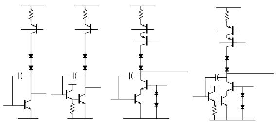
In between these two stages is a voltage-gain stage, usually a common-emitter stage with perhaps an emitter-follower buffer and/or a cascode connection. One can find its gain at low frequencies by the usual methods. This stage, however, almost always has a compensation capacitor connected between its input and output, as shown. Skipping the analysis (you can ask me...), the overall differential gain of the op-amp, at higher frequencies is given by:
