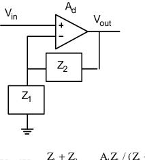
$$V_{out} / V_{in} = \frac{Z_1 + Z_2}{Z_1} \times \frac{A_d Z_1 / (Z_1 + Z_2)}{1 + A_d Z_1 / (Z_1 + Z_2)_1}$$
