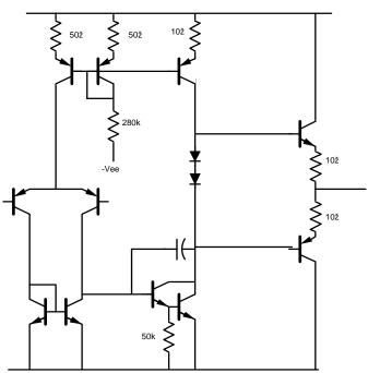
Above is one op-amp circuit. Several more are shown in a related hand-out. Most op-amps can be broken down into three parts: A differential input stage, a second voltage-gain stage, and an output buffer stage.
