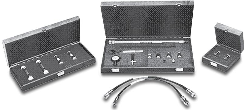
**Figure 1. Mechanical cal standards and cal kit**
