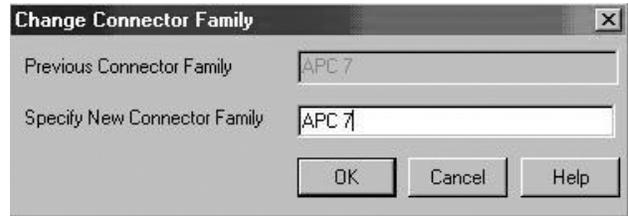
The cal kit's connector family can be renamed. The APC 7 connector family is being changed to 7mm.
