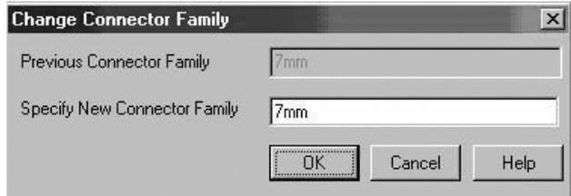
To set up a new kit, the connector family must be defined before adding calibration standards. Any changes to the connector definition must also be performed before editing the calibration standards.
