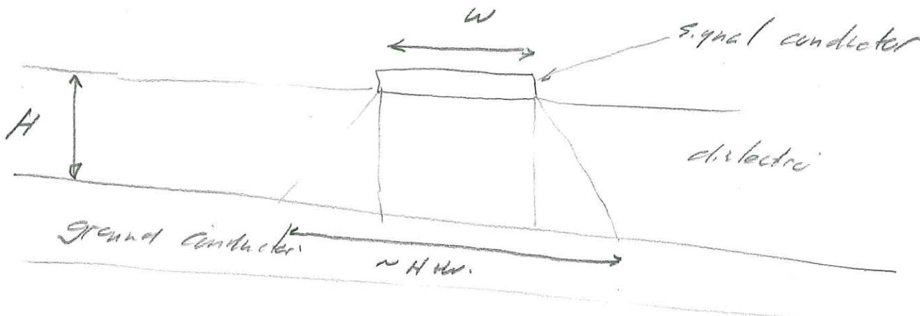
Now, the signal current is carried across the full conductor width  $w$ .
