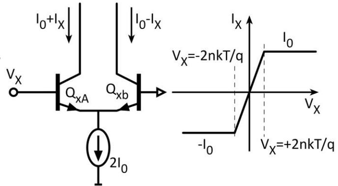
Problem 9 (218C only): Given the above models of the differential pair can you compute the phase/frequency detector voltage  $V_{DET}$  as a function of differential frequency  $\Delta\omega$ ?
