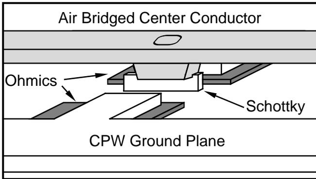
Figure 1: Perspective drawing showing the air bridged center conductor contacting the top of a diode. The Schottky contact is kept well away from the edge of the  $H^+$  implanted region, which ends outside the ohmics.
