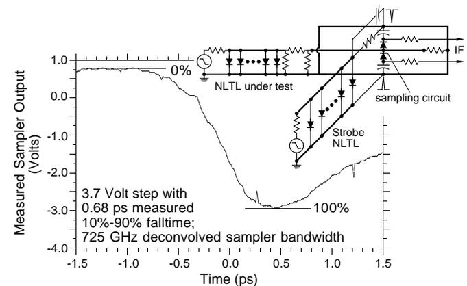
Figure 6: Measured output from a sampling circuit integrated on wafer with two NLTLs showing the  $0.68\text{ ps}$  step function. The inset shows a schematic diagram of the circuit.
