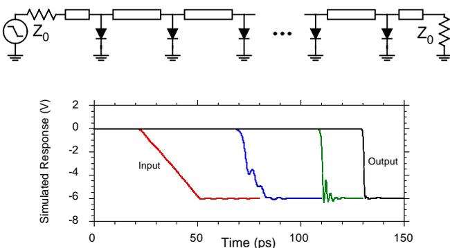
Figure 5: Schematic diagram of a nonlinear transmission line and a SPICE simulation showing the formation of a shock wave as a negative-going edge propagates down the line.
