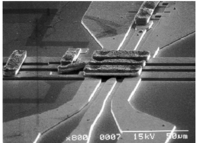
Figure 4: S.E.M. image of the sampling circuit and the output end of the NLTL that provides the strobe pulse to the two  $1\mu\text{m} \times 1\mu\text{m}$  sampling diodes.
