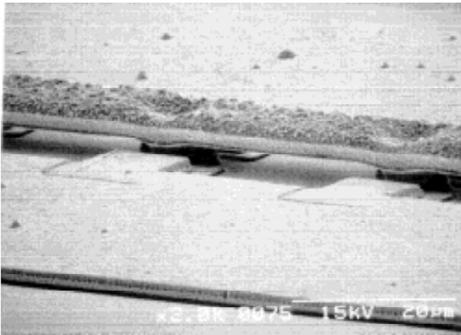
Figure 3: S.E.M. image showing the air bridged center conductor of the coplanar waveguide contacting the tops of the diodes on the NLTL without touching the substrate.
