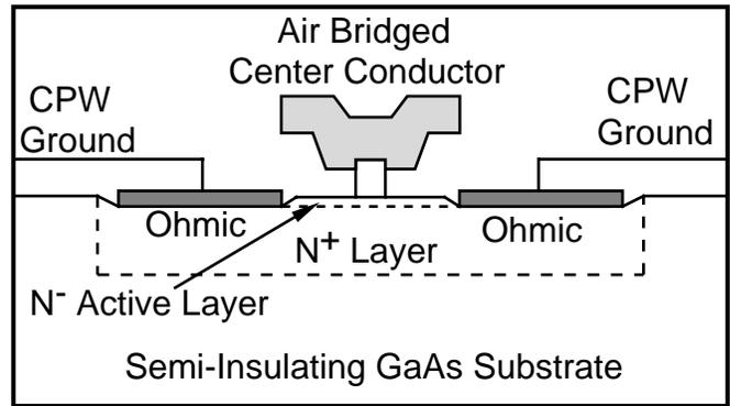
Figure 2: Cross section of the air bridge contacted diode. A layer of polyimide is used to keep the post off the substrate during electroplating. The ohmic contacts are recessed through the  $N^-$  active layer to a heavily doped  $N^+$  buried layer.
