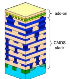
Illustration of 3D hybrid circuit: CMOS subsystem + nano-RRAM add-on
