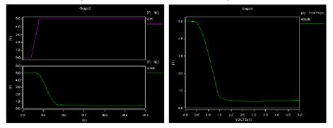
Type in "cscope" or "scope" to launch CosmoScope. Load your simulation results (inv.tr0 and inv.sw0), and you will see the corresponding waveform. Attach a screenshot of your waveforms in your lab report.
