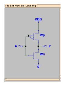
Voltage source, ground signal, pins and FETs can be found in the side toolbox:
