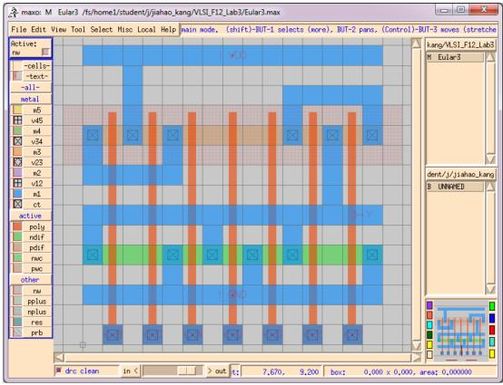
In this layout,  $\lambda$  is 0.15um, which means each track is 0.6um wide with 0.6um spacing.
