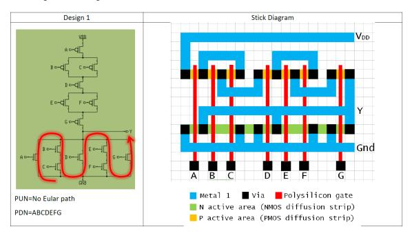
PDN has an Eular path ABCDEFG so that we arrange polysilicon gate colomns (poly) in sequence ABCDEFG. Hence, NMOS diffusion strip (ndiff) is uninterrupted. But PMOS diffusion strip (pdiff) will be definately interrupted no matter how poly are arranged.
