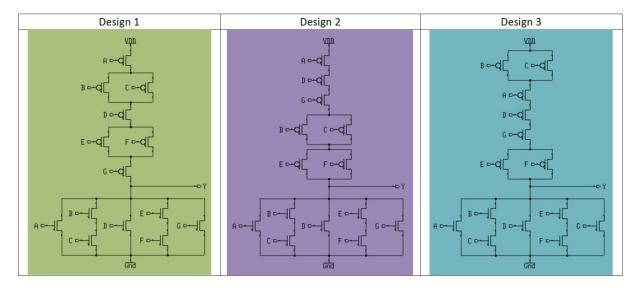
They all implement the function  $Y = \overline{A + BC + D + EF + G}$ , but I know there should be a best design (the optimum gate ordering), which would have the simplest layout and the smallest layout area.
