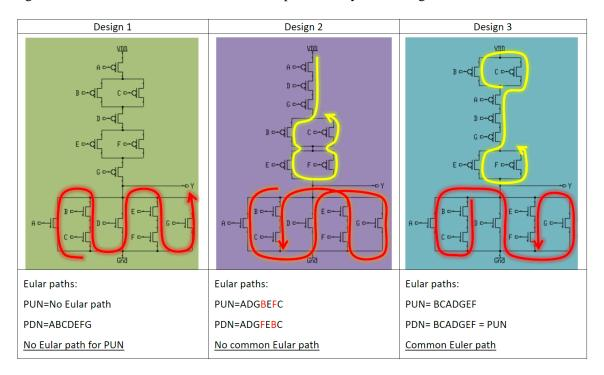
Finding a common Euler path in both graphs for the pull-down and pull-up net provides a gate ordering that minimizes the number of active-area breaks.
