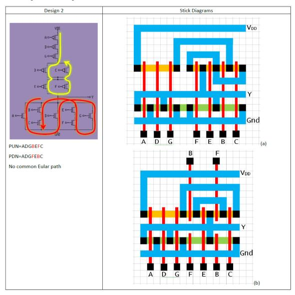
As we mentioned in Step 2, since Eular paths for PUN and PDN cannot be the same, we may have either <u>interrupted ndiff/pdiff with uninterrupted poly</u> (a) or <u>uninterrupted ndiff/pdiff with interrupted poly</u> (b).
