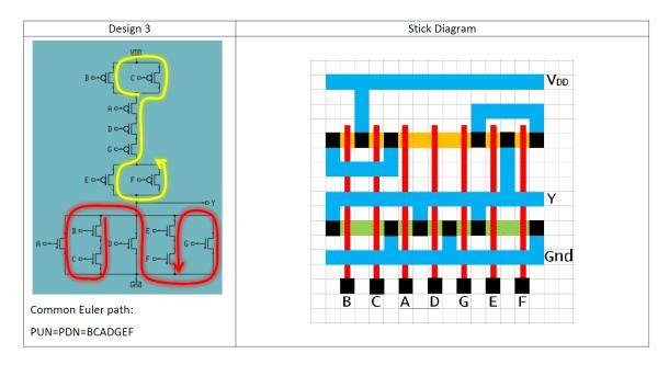
There is a common Eular path BCADGEF for both PUN and PDN. Hence, I arranged poly in ordering of BCADGEF and drew the stick diagram as shown above, which has <u>uninterrupted ndiff/pdiff</u> and <u>uninterrupted poly</u>.
