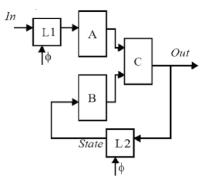
The L-units represent positive latches clocked by  $\phi$  (i.e., the latches are transparent when  $\phi$  is high). These latches have a setup time of 150 ps and a td-q delay of 250 ps (when the latch is transparent). The clock to output delay tclk-q is 120 ps, and thold is 110 ps. The clock has period Tclk and is high for a duration of  $T_{on}$ . In other words, the duty cycle of the clock is  $T_{on}/T_{clk}$ .
