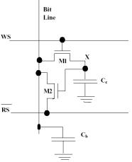
A generic SRAM cell is shown below. At first, it seems like the margins in such a memory cell should be good, since it contains two CMOS inverters, which we know have large margins. However, the problems are associated with those access devices connected to the cell. When cell is not accessed, it has great margins; when access devices are on, they act like load devices. Capacitance on bit lines is large enough to act like a voltage source.
