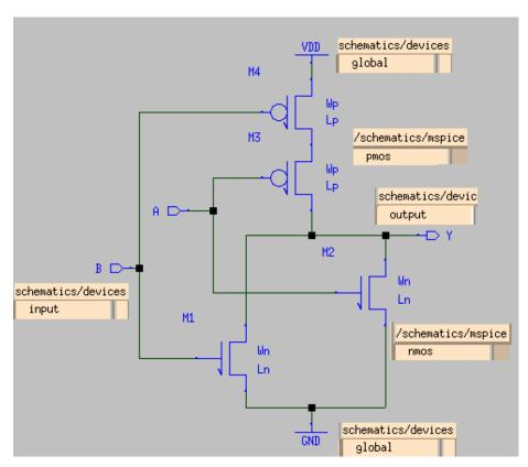
The models you will use are marked on the figure. You should give every model a name by double clicking on it. Note that you can modify the sizes of MOSFETs by double clicking on the symbol:
