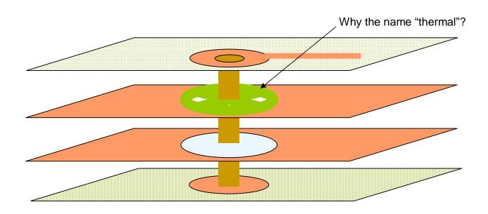
Thermal aperture shown highlighted ... actually it is copper (ORed-in with "+" plane)
