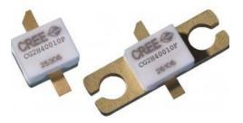
RF power amplifier will be designed around the Cree CG2H40010. The design and fabrication may be undertaken by students with an interest in RF power amplifier design, or a Cree reference circuit board may be obtained for inclusion in the platform. A pre-amplifier will be required to drive the Device Under Test. This can either be designed using a Cree device, or investigated and selected from commercially available options.
