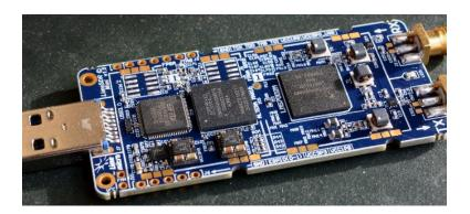
Group will investigate and select the digital hardware and transceiver for to implement the digital predistortion system. An example of open source support hardware is the LimeSDR mini platform.
