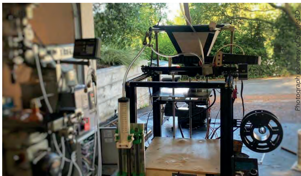
Over the summer, the members of Spinjet3D built a prototype of their printer to test different binder solutions.
