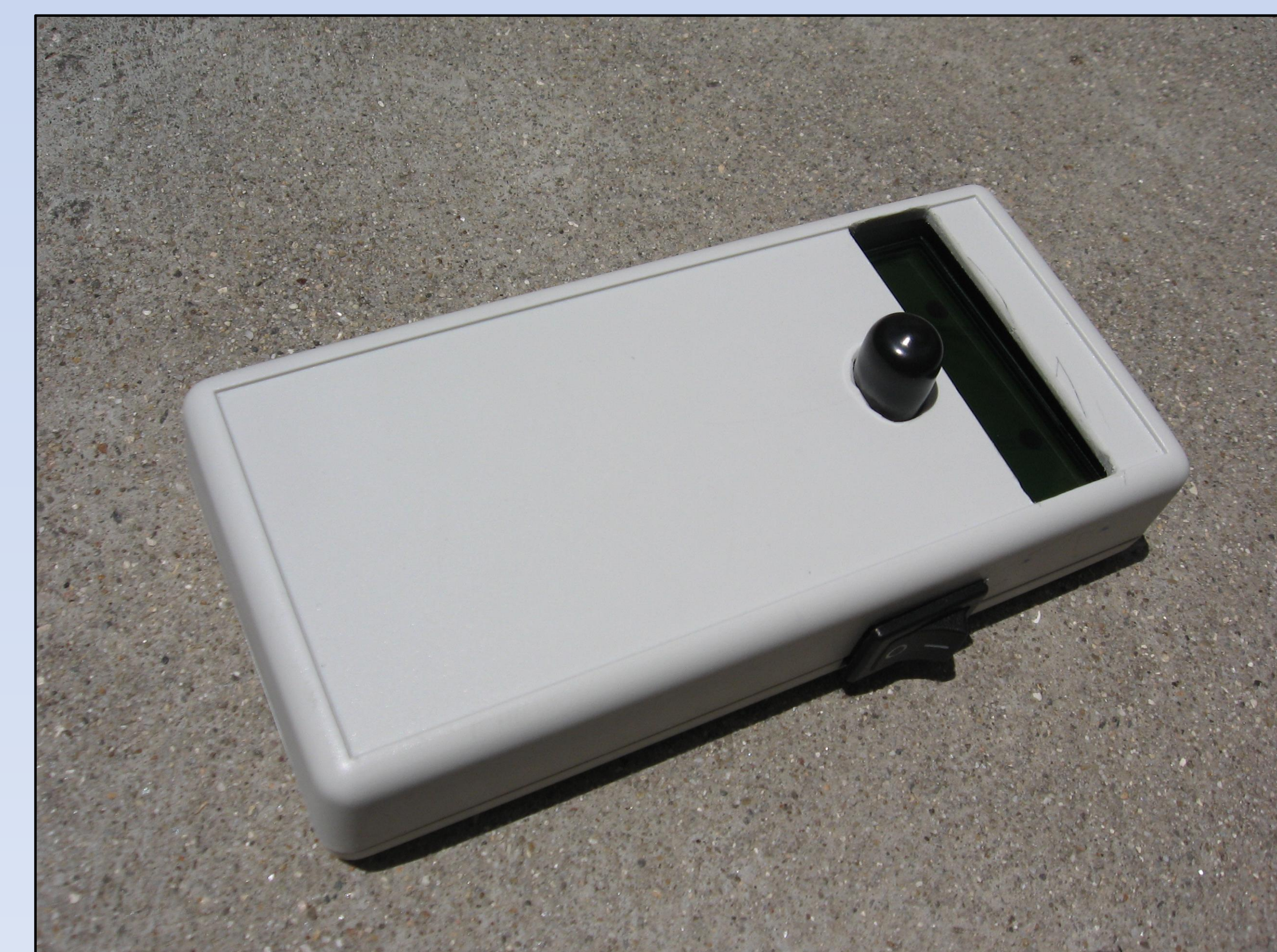
Above: Enclosure with LCD display and 4-directional switch for user interface Left: Internal Circuitry
