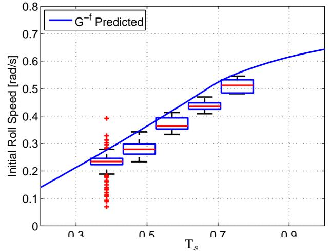
Fig. 6.  $G^{-f}$  timing map above is calculated running isolated frontal simulations such as those shown in Fig. 5. The full 3D dynamic simulation is represented with the box and whisker plots. The box is the 25-75% interval, while the bars represent the 9% to 91% interval. Outliers are plotted with red crosses and we suspect they are more prevalent at shorter time steps due to the larger amount of gaits. The frontal plane system behaves overall very similarly to the full 3D dynamical system.
