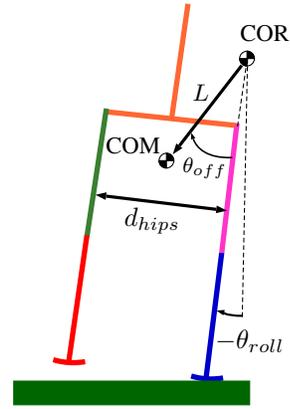
Fig. 4. Each foot has a Center of Rotation (COR) in placed directly above their respective hip. The system behaves very similarly to a stable pendulum with length  $L$ . Only there is a pendulum offset  $\theta_{off}$
