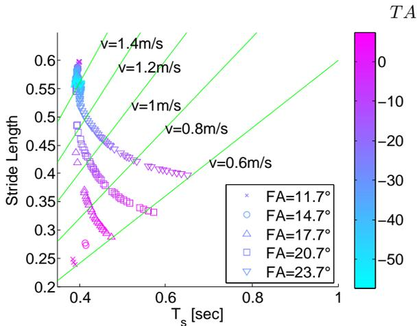
Fig. 3. This figure depicts the gait space spanned by  $G_s$  through the variation of two control reference parameters  $FA$  and  $TA$ . The gait characteristic is at the steady fixed point of the controller on flat ground. The green lines are provided as reference for isocurves of constant forward velocity.
