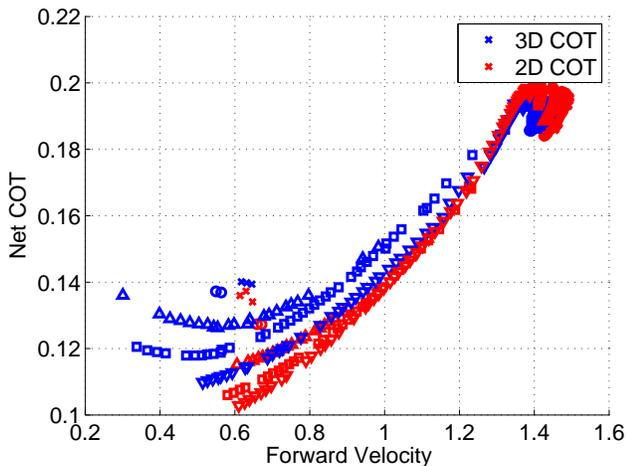
Fig. 11. Cost of Transport corresponding to Eq. 25. Note that in general faster walking speeds correlated with more energy expenditure for the 2D gaits. Remembering that adding the frontal plane dynamics for 3D walking results in energy efficient gaits at shorter stride time (as seen in Fig. 7), we can explain the more efficient 3D walkers at higher speeds (1.2 to 1.5 m/s). The faster walking gaits corresponded gaits corresponded to short stride times of .35 to .4 [s] (Fig. 3)
