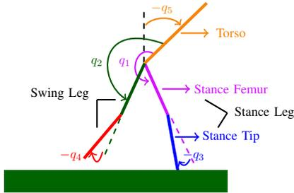
Fig. 2. Diagram of the robot from the sagittal plane
