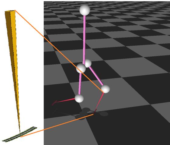
Fig. 1. The Visualization from MuJoCo Simulator is on the right. We placed a magnified view of the curved foot geometry on the left. The center of curvature 80cm above the foot, arc length of  $10^\circ$ , and a width of 1.8cm
