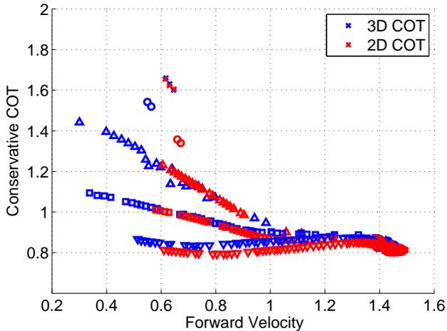
Fig. 10. This COT corresponds to the work in Eq. 24. Interestingly, the conservative COT is not correlated with the trend of the net COT. We suspect the accelerating and decelerations of the legs during the gait slower gaits greatly penalizes the gait. The effect of the frontal plane dynamics appear to be negligible.
