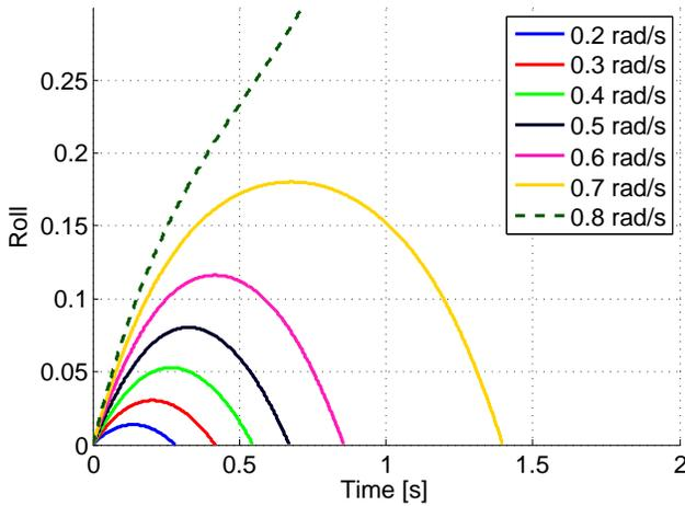
Fig. 5. To determine times of return the model was simulated with various initial roll speeds. The dashed line signifies an initial roll speed in which the robot tips over. Since this trajectory never recovers to  $\theta_{roll} = 0$ , the time return map is undefined for this velocity.
