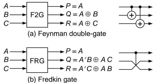
**Fig. 2. Parity-preserving reversible gates, satisfying  $A \oplus B \oplus C = P \oplus Q \oplus R$ : Block diagrams and symbolic forms.**
