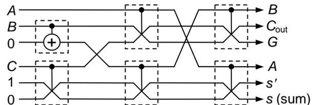
**Fig. 3. Binary full-adder built of Fredkin gates. The single Feynman gate fans out B.**
