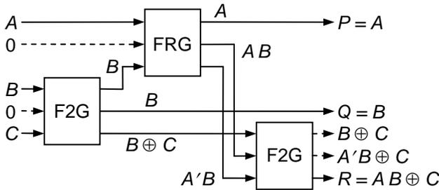
Fig. 5. Synthesizing a TG from one FRG and two F2Gs, with parity preservation.
