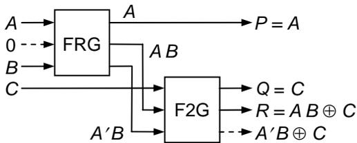
Fig. 6. Synthesizing a TG-like element from one FRG and one F2Gs.
