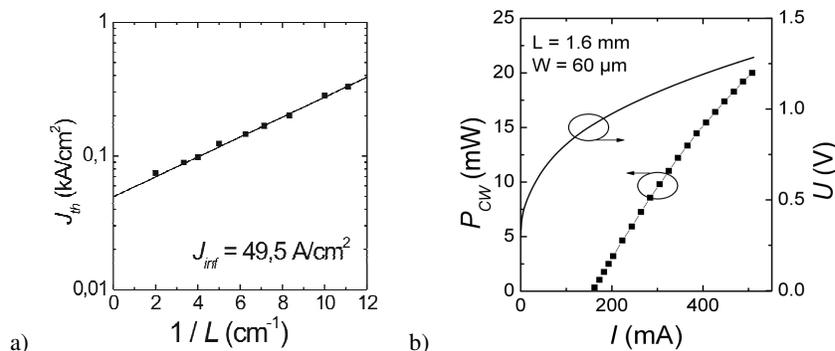
Fig. 2. a) Threshold current densities over the inverse length. b) Power over current and voltage over current characteristics of the  $2.65 \mu\text{m}$  laser.
