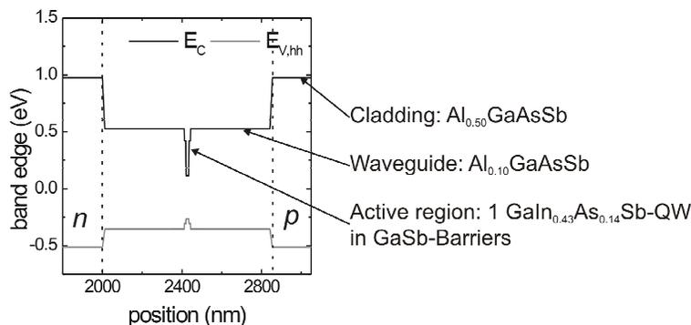
Fig. 1. Schematic energy-band diagram of the 2.7  $\mu\text{m}$  edge emitting laser
