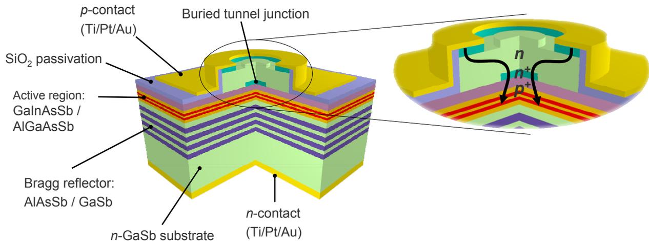
Figure 3. Schematic structure of the gain mirror. Carriers are injected into the active region through the top and bottom contacts. The carriers are confined to the center of the device by means of the buried tunnel junction.
