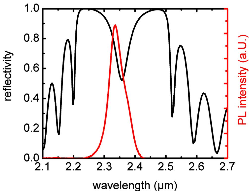
Figure 4. Reflectance spectrum and photoluminescence curve measured from the sample.
