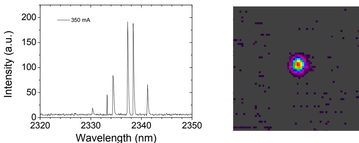
Figure 8. Left: Optical spectrum from the  $60\ \mu\text{m}$  component at  $350\ \text{mA}$  current. Right: Beam profile of the  $60\ \mu\text{m}$  component measured with a pyroelectric camera. Exposure time 10 frames.
