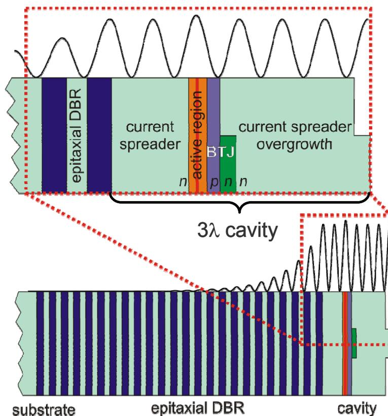
Figure 1. Field distribution in the GaSb-based gain mirror. The structure consists of an epitaxial GaSb / AlAsSb mirror and a  $3\lambda$ -thick layer structure on top including the active region in an antinode and the BTJ in a node of the optical field.
