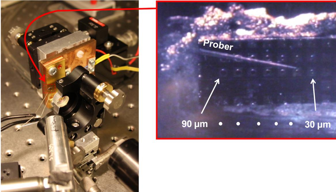
Figure 5. *Left*: A photograph of the laser. *Right*: Soldered semiconductor chip with different components having aperture diameters varying from 30  $\mu\text{m}$  to 90  $\mu\text{m}$ . The probe is contacted to the 40  $\mu\text{m}$  device.
