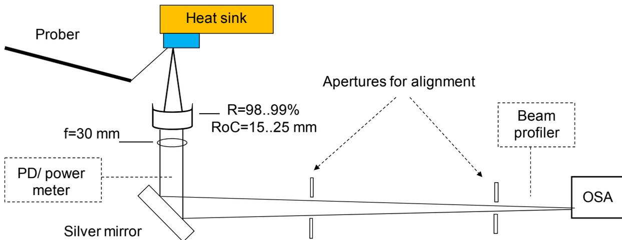
Figure 6. Schematics of the laser characterization setup. PD=Photodiode, OSA=Optical spectrum analyzer
