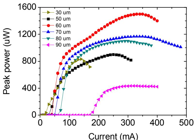
Figure 7. Light output characteristics from different components using 99% reflective output coupler.
