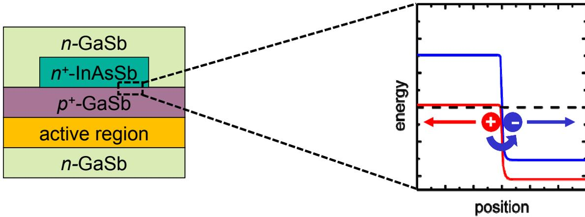
Figure 2. Schematic structure of the tunnel junction serving as a current aperture, and the band diagram of the p<sup>+</sup>-GaSb / n<sup>+</sup>-InAsSb heterojunction, where the tunneling occurs. On the etched outer parts of the aperture, a blocking p<sup>+</sup>- / n-GaSb structure is formed.
