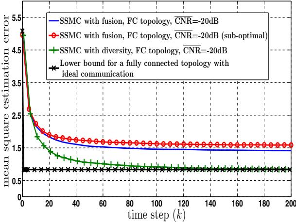
Fig. 2. A comparison of fusion and diversity techniques for the SSMC case with  $M=6$ , the graph is fully connected with fading channels for non-ideal communication cases.
