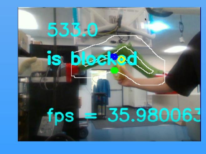
Our program can detect objects around the outer layer of the robotic arm. When the program identifies the objects that could cause collision, it sends a 'blocked' signal. To raise the performance of collision avoidance, our camera tracks the center of arm, indicated by the yellow circle in the center of robotic arm
