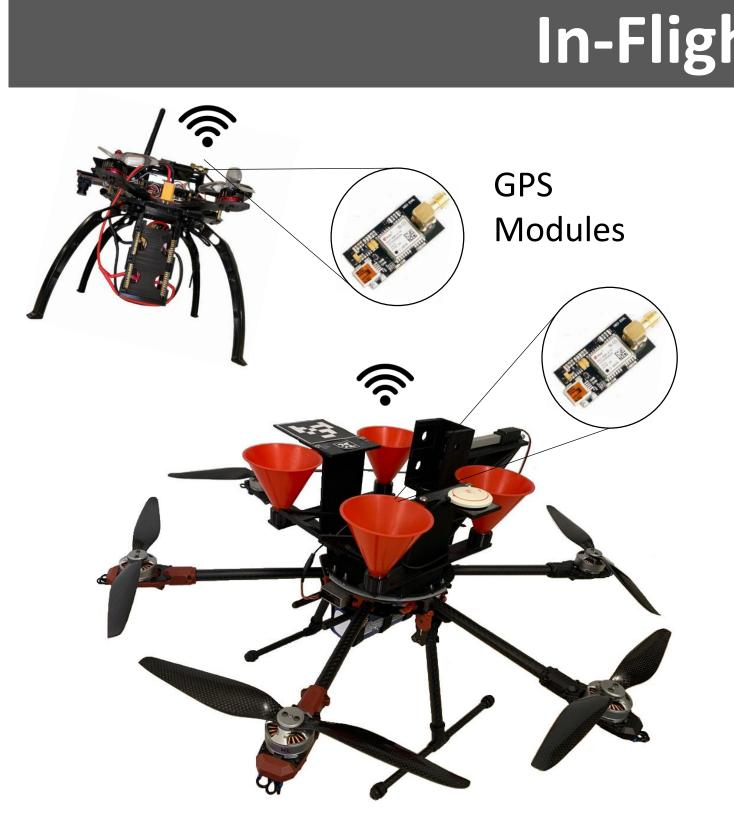
Waypoint Navigation The tanker communicates its coordinates to the receiver over WiFi. Using centimeterlevel accurate Real-Time Kinematics present on both drones, the receiver drone navigates to and hovers 6 feet above the tanker.
