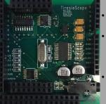
Compatible with standard Arduino shield footprint Contains the audio codec and the other components required to generate audio on the stereo jack Includes connections for the sensors
