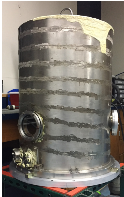
Figure: Bell vacuum chamber for testing
