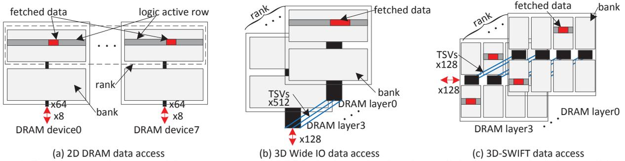
Figure 1: Data access mechanisms in different memories. (a) DDR3: the data is distributed over all devices in a rank. Only a small fraction of row is fetched in each memory access; (b) Wide IO: the data is placed in a large row and no individual device exists. Still only a portion of data is fetched; (c) 3D-SWIFT: the width of fetched data matches cacheline width. The rest of a row is idle.
