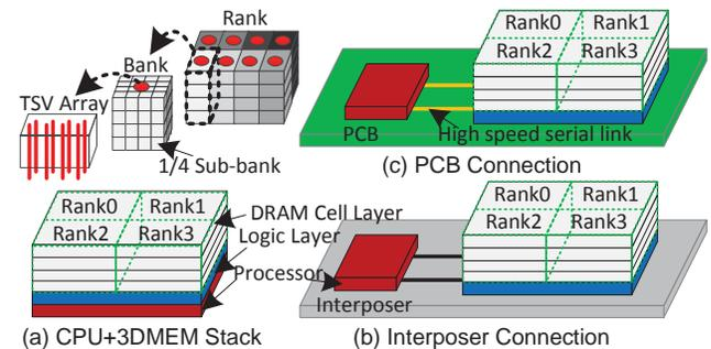
Figure 3: 3D-SWIFT memory subsystem and possible applications. (a) 3D-SWIFT directly stacks on the top of CPU; (b) 3D-SWIFT is connected to CPU by interposer; (c) 3D-SWIFT is placed on PCB with high speed links. Multiple 3D-SWIFTs can be populated to provide large memory capacity (not shown).
