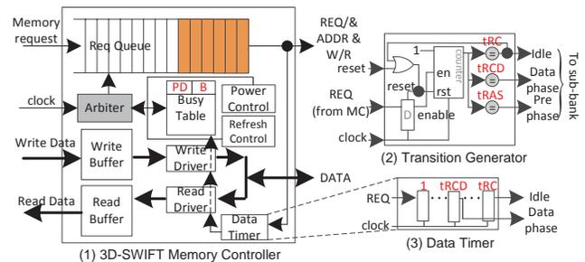
Figure 5: Memory controller design in 3D-SWIFT. (1) Memory controller; (2) Transition generator; (3) Data timer. The length of the counter and shifter are determined by the cycle number of  $t_{RC}$ .
