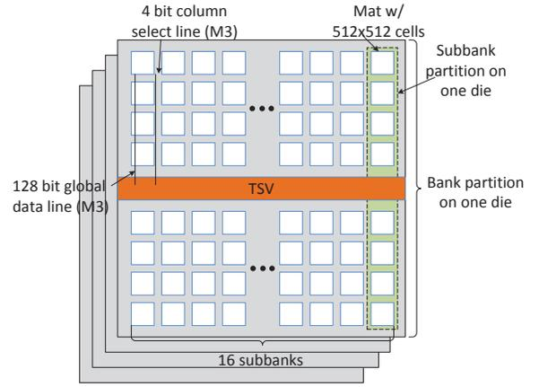
Figure 6: The Floorplan of 3D-SWIFT. A sub-bank consists of 32 mats and each mat is 256Kb (512 $\times$ 512).
