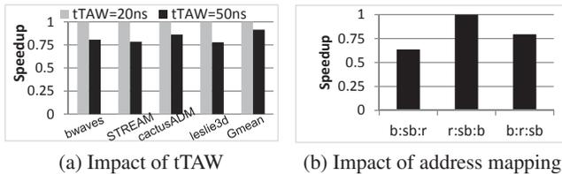
Figure 8: Sensitivity Study. (a) Impact of tTAW; (b) Performance with different address mapping schemes. “r”-row, “b”-bank, “sb”-sub-bank.
