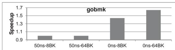
Figure 2: The impact of power constraint on 3D DRAM. The simulation is done with 8/64 banks (BK) and tTAW=50ns/0ns (see Section 5 for the details of simulation setups).
