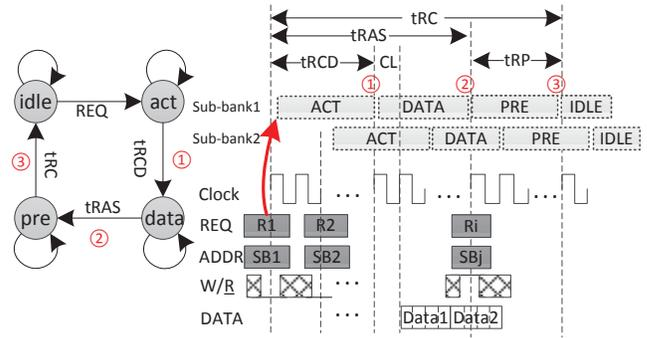
Figure 4: Packet-based interface protocol. Memory controller only issues REQ to initiate a memory access. The sub-bank can complete the data transfer and precharge to close the row automatically.
