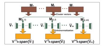
Fig. 2. Projection matrix construction in BDSM . In this figure,  $M_j = ((s_0C - G)^{-1}C)^{j-1}(s_0C - G)^{-1}B$ ,  $j = 1, \cdots, l$ . The *i*-th columns of  $M_j$ 's are grouped to form  $\bar{V}_i$   $(i = 1, \cdots, m)$ . And then  $V_i$  is computed such that  $V_i = \bar{V}_i$ , for  $i = 1, \cdots, m$ . Note that, in PRIMA the projection matrix for (1) is constructed without clustering, such that  $V = \text{span}\{M_1, \cdots, M_l\}$  with more computational cost.
