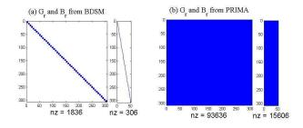
Fig. 4. The matrix structures of ckt1's ROMs, obtained from BDSM and PRIMA, respectively.
