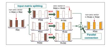
Fig. 1. The BDSM model reduction scheme for a linear network with m input ports, which is based on column-by-column moment matching. After input matrix splitting, the original model is decomposed into m MIMO subsystems. Then using the projection process,  $H_{ir}(s)$  captures the first l moments of H(s)'s *i*-th column. Finally, the parallel connection of all ROMs guarantees the preservation of H(s)'s first l moments.
